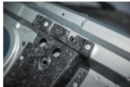
**2016 BMW 7 SERIES (G12)** inner quarter reinforcement CFRP
