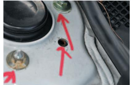
**MISALIGNED** strut mounting bolts
