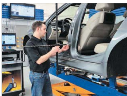
Car-O-Liner's 3D measuring tool
